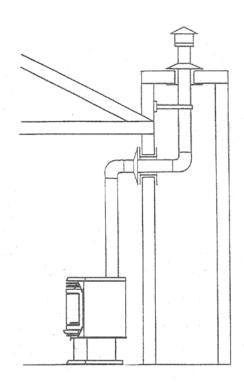
For best venting performance, we recommend total vent height of 10 ft (3m) to 30 ft (9m). Total horizontal length depends on the number of elbows used. The venting
